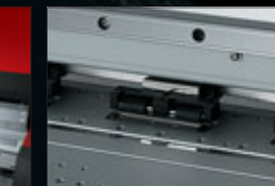
New media feed system includes 16 pinch rollers for letter perfect printing during high-volume runs
